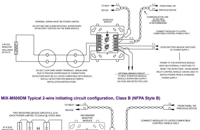
ALL WIRING SHOWN IS SUPERVISED AND POWER LIMITED.
