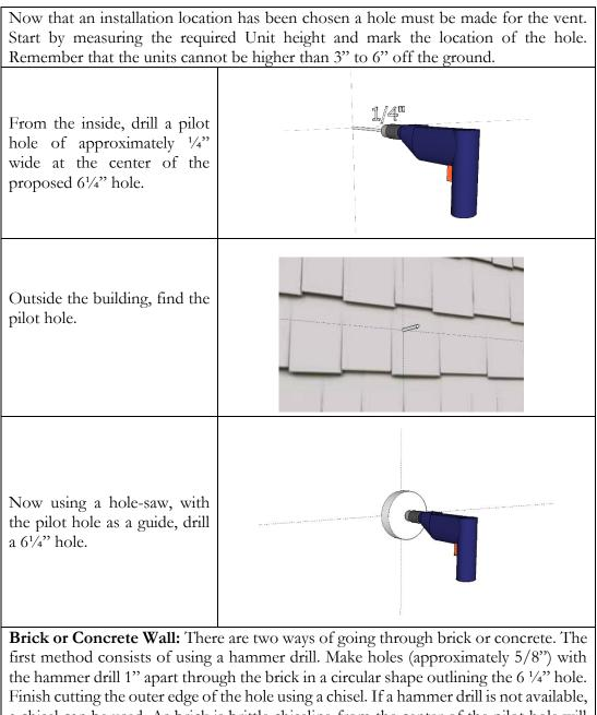
a chisel can be used. As brick is brittle chiseling from the center of the pilot hole will chip the brick easily. Continue chiseling until you reach the outer edge of the 6 1/4" hole.
