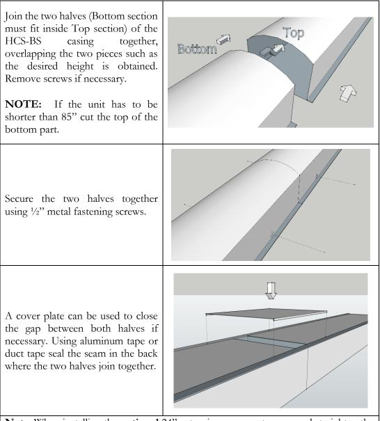
**Note**: When installing the **optional** 24" extension, remove top cap and straighten the 90° elbow. Use the 6" galvanized pipe to extend the length needed. Cut the pipe to the proper length before snapping it together. Attach the top cap to the extension cover with the 4 screws provided. Add exterior cover to the base and fasten securely with the provided screws.
