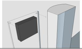
Replace the front of the unit using the 4 Screw Caps with the 4 original screws.
