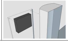
With the help of a tie wrap attach the flex pipe to the collar on the back of the unit before attaching the unit to the wall. Insert the other end of the flex pipe inside the hole in the wall. (a few Small 9/16" Screw can be used to affix the flex to the mount)
