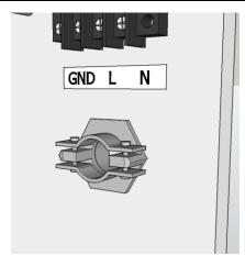
Once the wire has been run through the plate, you must connect the wire to the unit matching the colors of the inside wires. After the wiring has been completed, you can attach the small cover plate to the back plate and return to the original installation procedures.
