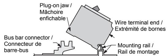
**NOTE:** When using QO tandem circuit breakers with the plug-on neutral (PON) loadcentres, use only Series 3 or higher. The Series of the tandem breaker is indicated on the side cover of the breaker as well as the breaker carton label.
