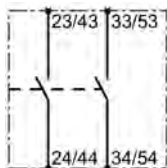
Auxiliary switch block, lateral, 2 NO contacts
