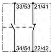
Auxiliary switch block, lateral, 1 NO contact, 1 NC contact
