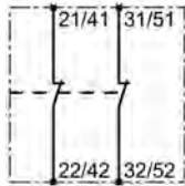
Auxiliary switch block, lateral, 2 NC contacts
