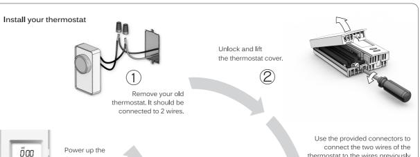
thermostat to the wires previously thermostat. (5)connected to your old thermostat.
