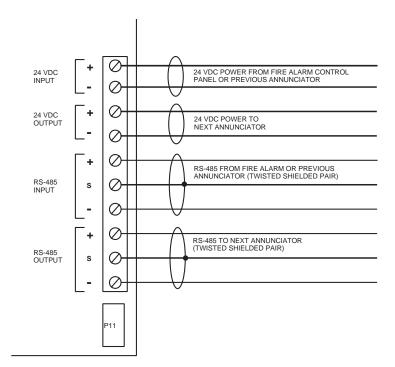
RS-485 output terminals. This is removed on all except the last wired module.
