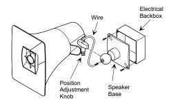
Figure 2 - Mounting to an Electrical Backbox
