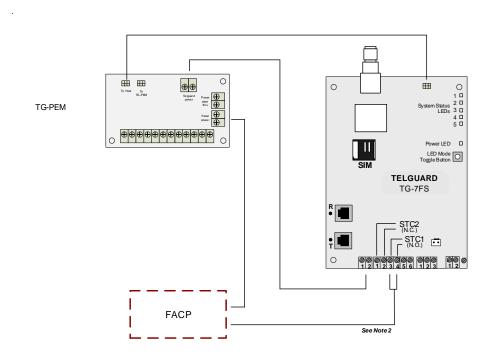
UL/ULC Compliance Note 2: STC1 needs to be connected to a panel input zone to indicate all trouble conditions.
