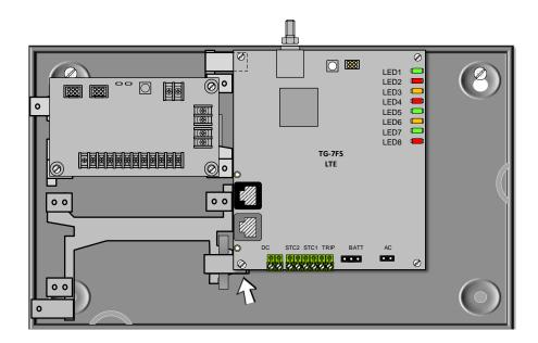
Use the three provided TG-PEM mounting screws to secure the second TG-PEM circuit board onto the bracket.
