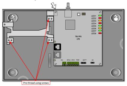
• Use the three provided mounting screws to secure the TG-PEM board onto the bracket in the holes that you pre-threaded.
