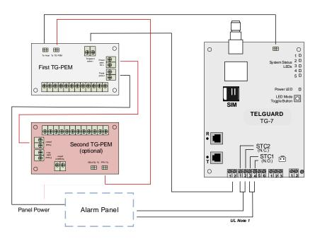
UL/ULC Compliance Note 1: STC1 needs to be connected to a 24-hour panel input zone to indicate alarm conditions from TG-PEM. STC2 could be used to indicate TG-7FS or TG-7FE trouble conditions.
