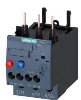
Overload relay 11...16 A Thermal For motor protection Size S0, Class 10 Contactor mounting Main circuit: Screw Auxiliary circuit: Screw Manual-Automatic-Reset
