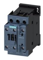
power contactor, AC-3e/AC-3, 17 A, 7.5 kW / 400 V, 3-pole, 220 V AC, 50 Hz / 240 V, 60 Hz, auxiliary contacts: 1 NO + 1 NC, screw terminal, size: S0
